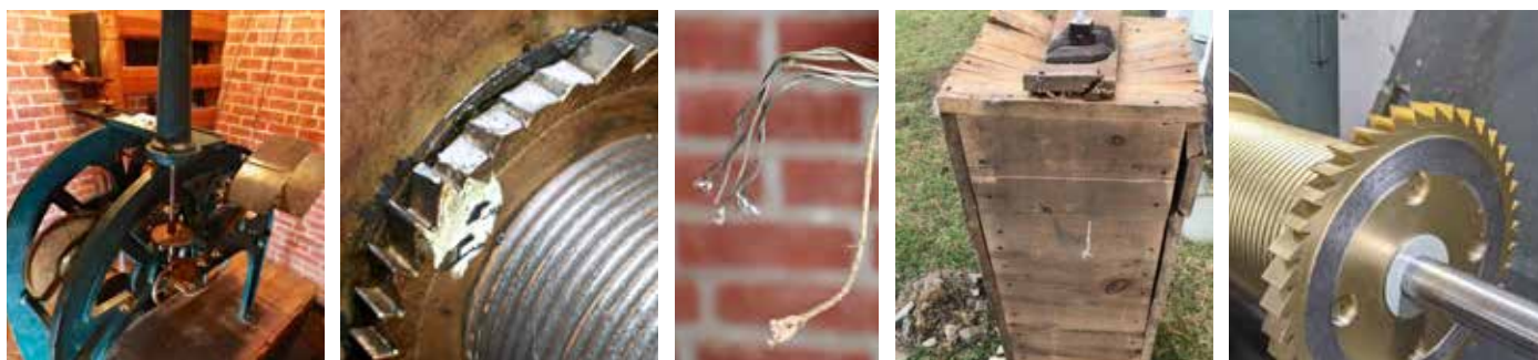
Clock frame & gear housing, broken ratchet wheel, snapped steel cable with hemp rope, damaged weight box, newly milled ratchet wheel & drum
