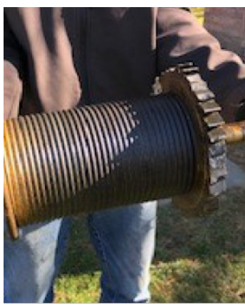
Broken ratchet wheel and drum removed for repair
